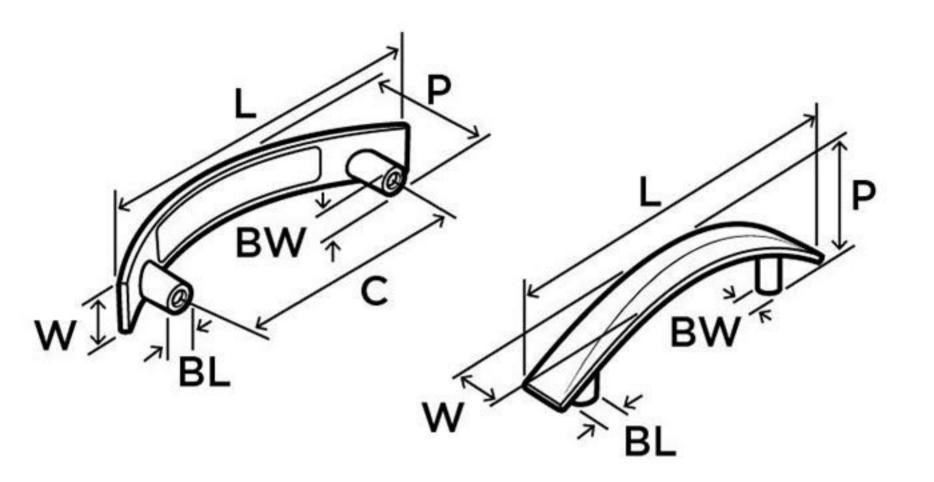
L (Length) = 4-1/8in(105mm)W (Width) = 11/16in(17mm)
