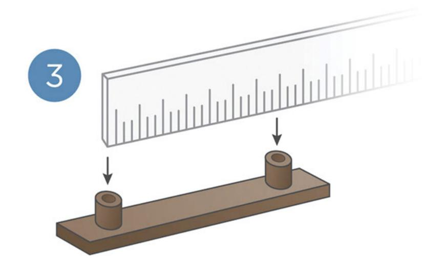
MAKE SURE THE CENTER TO CENTER DIMENSIONS OF THE CABINET PULL MATCH THE SCREW HOLE DIMENSIONS
